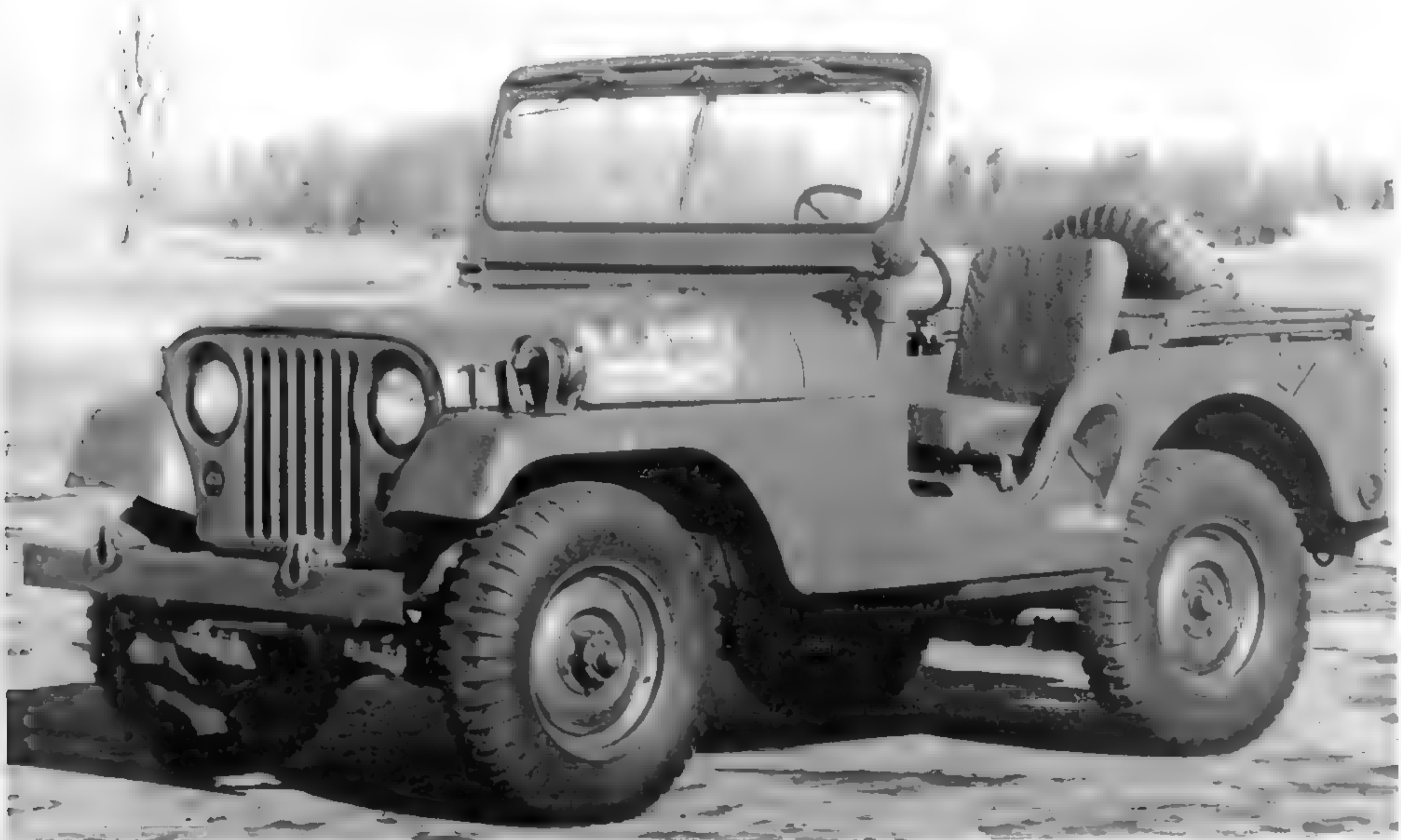
Along with the more powerful F-head engine, other improvements were introduced that made the M38A1 only vaguely resemble the M38. Among the changes was a reshaped hood. (U.S. Army photo)
